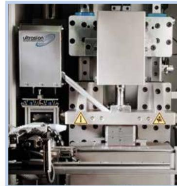
The technology uses standard room temperature pellets which as they are melted and injected in one process eliminates residence time and therefore eliminates material degradation.
