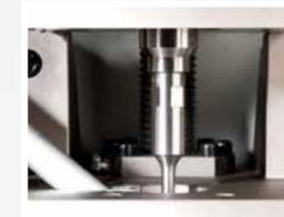
Reduced material viscosity also means that the molding pressures required are much reduced over traditional micro molding technologies, typically in the range of 300-500 bar as opposed to the 1500-2000 bar that molders are used to.
