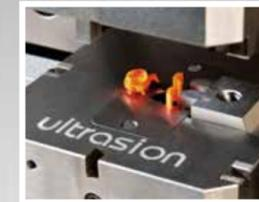
Plastic melted through the use of ultrasonics exhibits radically different and advantageous characteristics when compared with plastics melted through the use of traditional heater bands.
